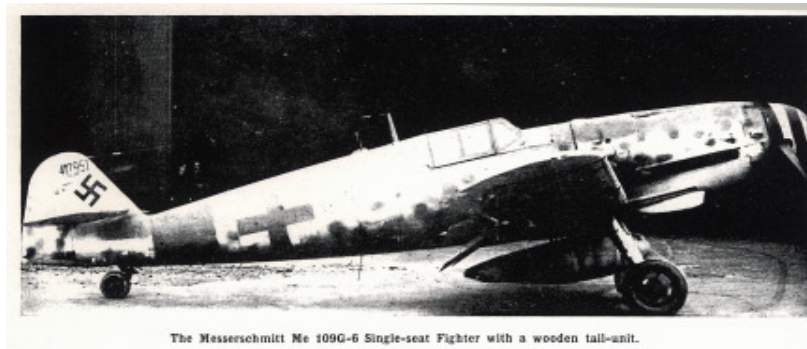
The Messerschmitt Me 109G-6 Single-seat Fighter with a wooden tail-unit.
